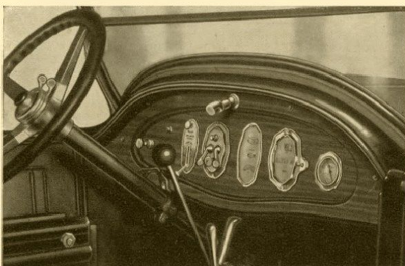
This view shows the new walnut instrument board with recess for instruments. Note the commodious driving compartment and the convenience of all levers and pedals.
