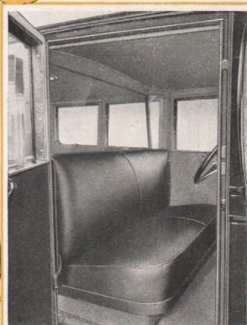
Front Compartment of the Enclosed Drive Limousine. Glass partition dividing front and rear compartments is lowered into section behind front seat
