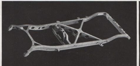
RIGID-X FRAME! A new kind of Double drop frame construction. Stronger, stiffer, to withstand twisting strains. Low to the ground for greater Safety and Riding Comfort.
