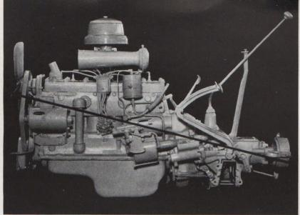
IT'S A FLOATING POWER SIX! The engine is suspended in balance, at just two points, on cushions of rubber. It dissipates its own vibration. The famous Plymouth smoothness! Floating Power means a more restful ride—and longer life for your car.
