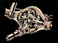
REAR AXLE — The new "Square" Hypoid fully floating asle with Banjo type housing incorporating a welded back cover for rigidity and strength. The crown wheel assembly is withdrawn as a unit through the forward inspection cover.
