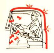
NEW COMFORT SEATING FOR THREE. A combination of moulded foam rubber and a shaped metal basepan forms the basis of the Trader's new type of seating. It holds the driver in a relaxed position, virtually eliminating the bounce associated with the normal spring type seat and which is especially noticeable on unladen trucks. The dual passenger seat is
