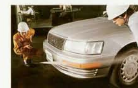
Top and second photos: two LS 400 styling models show different front-end treatments considered. At left, the Lexus wind tunnel; above, an LS 400 in the tunnel during aerodynamic testing.
