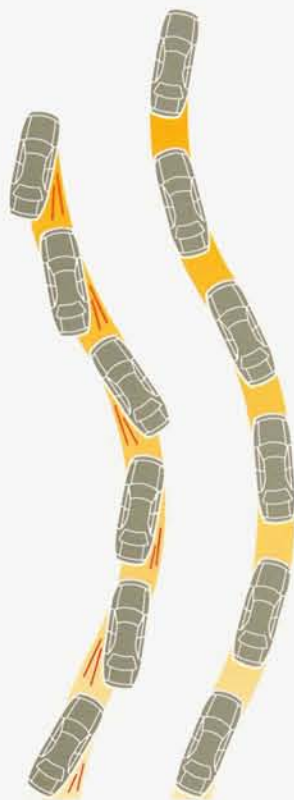
With the Traction Control system, control of the car under slippery road conditions is greatly improved (path at right).
