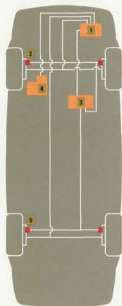
Antilock braking system (ABS) consists of wheel-speed sensors, a tiny special-purpose computer and a hydraulic control unit.
