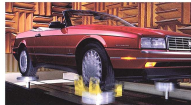
The road simulator demonstrates how the Road-Sensing Suspension isolates the Allanté from major road disturbances. Road-Sensing Suspension actually reads the road one inch at a time at 60 mph and adjusts each wheel accordingly.
