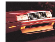
The front air dam of the 1993 Allanté manages airflow under the car, and aids stability at higher speeds typical of international driving conditions.
