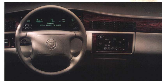
The digital instrument cluster of DeVille is now enhanced with an electronic, digital gear selection indicator.
