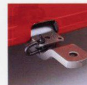
Standard Towbar* Rated at 1200 kg for manual vehicles and 1600 kg for auto.
