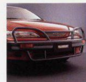
'Smart' Bull Bar Designed to be compatible with the airbag system and comply with current Australian Design Rules.
