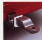
Heavy Duty Towbar* 2300 kg towing capacity with the aid of hitch and load levelling device (purchased separately).
