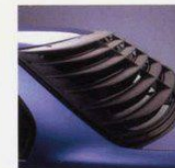
Rear Louvre (sedans only) Unique Ford design protects rear seat passengers from the harsh Australian sun and helps to reduce glare.
