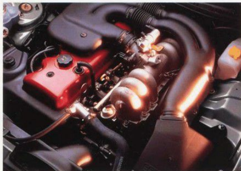
▲ 4.0 MULTIPPOINT EFI (FAIRMONT GHIA). Bore & stroke mm 92.26 x 99.3 Cylinder head OHC Aluminium alloy Displacement cc 3984 Compression ratio 9.3:1 Air induction Dual resonance intake manifold Fuel System Elect. multipoint fuel inject. controlled by EEC-V Engine Management System Fuel Regular Unleaded Max Power DIN kW/rpm 164/5000 Max Torque Nm/rpm 366/3150
