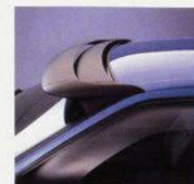
Front Sunvisor Fitted externally to the top of the windscreen to provide protection from the glare of the sun for safer driving.
