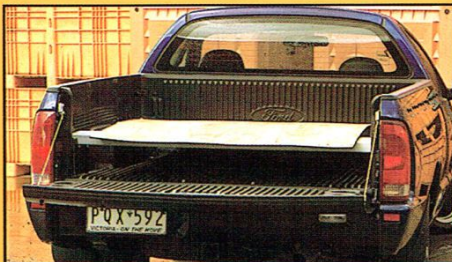
SSB loadbed. Load divide flexibility using two timber pieces & a building sheet. Load bed divided horizontally into two load areas.
