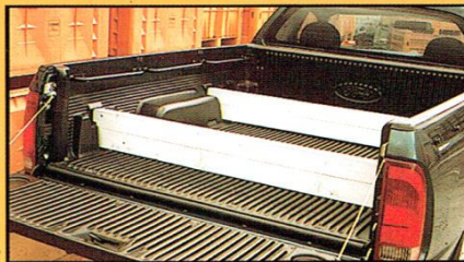
SSB loadbed. Load divide flexibility using two timber pieces. Load bed divided vertically into three load areas.
