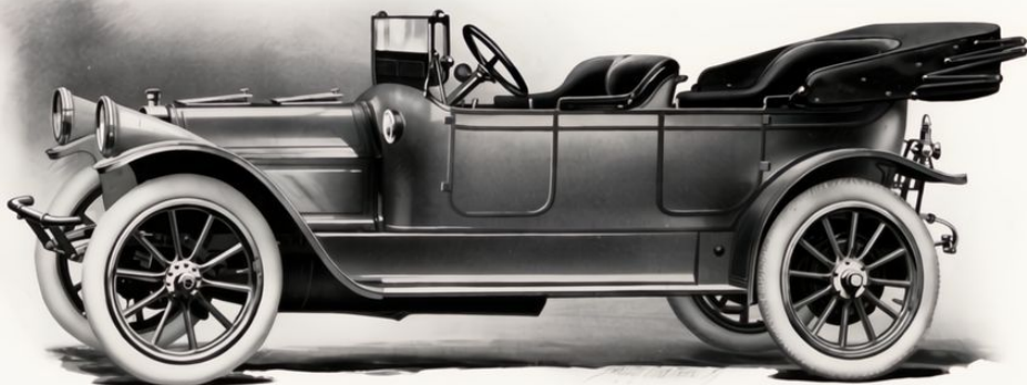
38 Horse-power, Six-cylinder Pierce-Arrow Touring Car, Model C2, seating four persons
