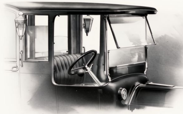
Brougham Detail, showing "Clear Vision" Glass Front
