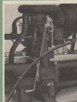
The Automatic Choke . . . a new Pierce-Arrow development . . . feeds the engine a perfect cold-starting mixture, and prevents "flooding".
