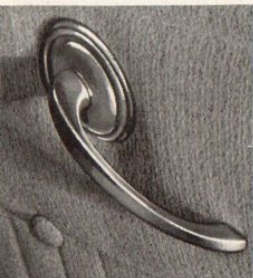
DOOR HANDLES, inside and out, curve inward for greater safety.
