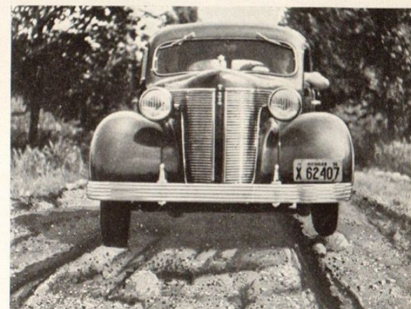
INDEPENDENT FRONT SPRINGS, permit wheels to follow the road, yet bodies stay level.
