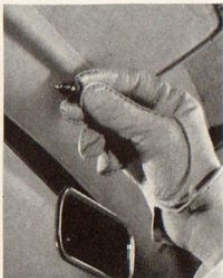
EVEN THE windshield wiper knob is soft rubber, for protection.
