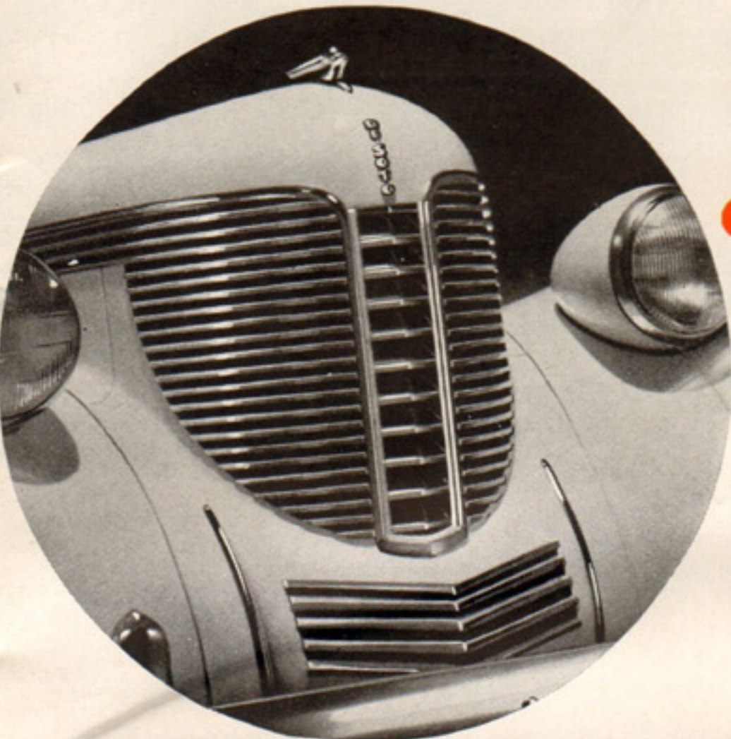
THIS CHROMIUM, die-cast radiator grille symbolizes the smart, modern styling of this great new De Soto. Notice how all contours are smoothly streamlined.
