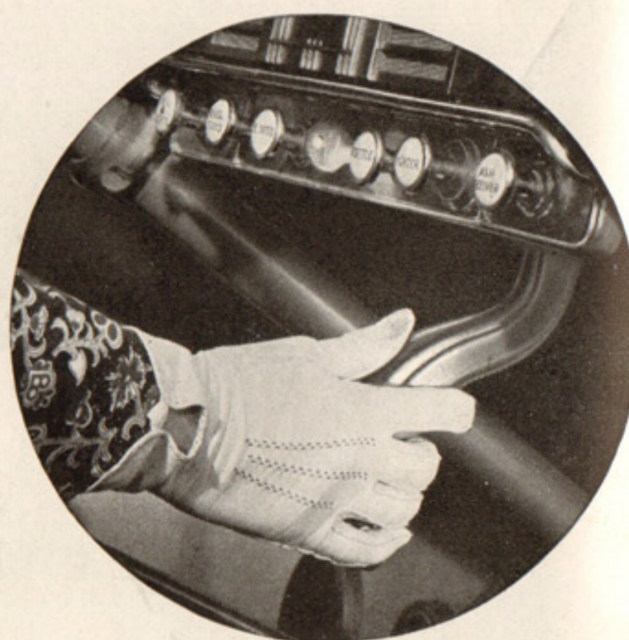
THIS "PISTOL-GRIP" parking brake is off the floor—providing more leg room.
