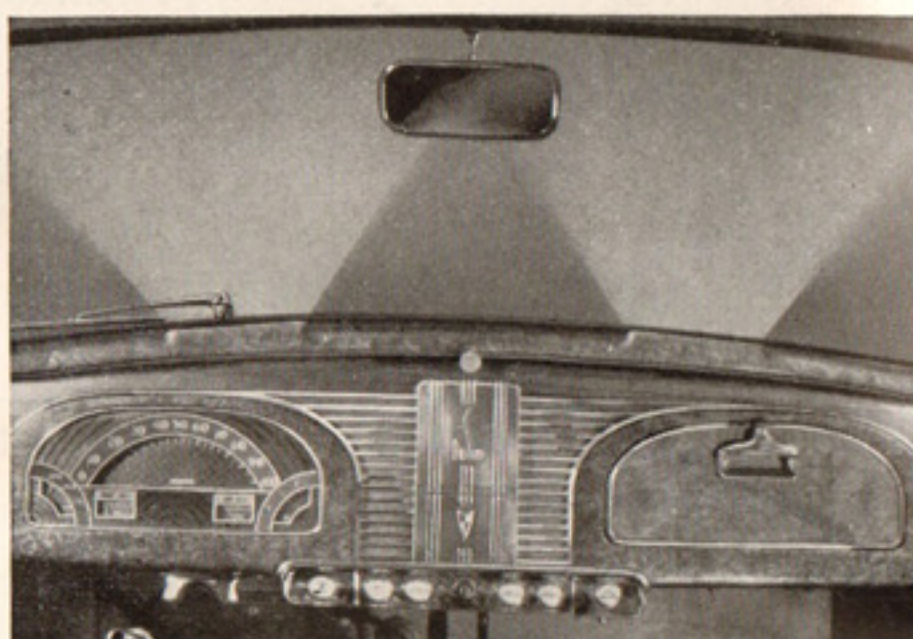
BIGGER DEFROSTER VENTS are built in at either end of the instrument panel and, when attached to a car heater, keep the windshield clear in stormy weather.
