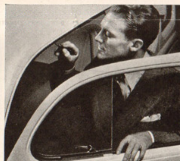
LAUGH AT RAIN and dampness! Drip moldings above doors catch rain, keep you dry.
