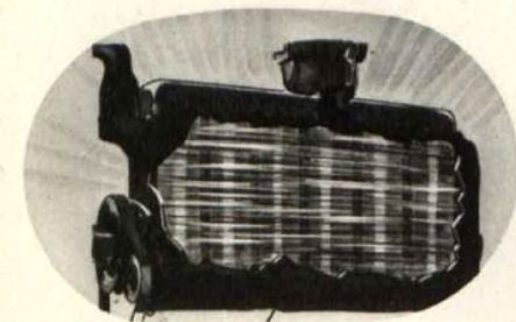
Full-length water-jacketing is an expensive car feature, but every Nash cylinder is so protected. Prevents uneven heat expansion . . . lowers oil temperature, lengthens engine life.
