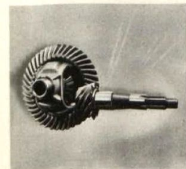
Hypoid gears in the rear axle, with taper roller bearings, add longer life; permit a lower center of gravity. Nash quality.
