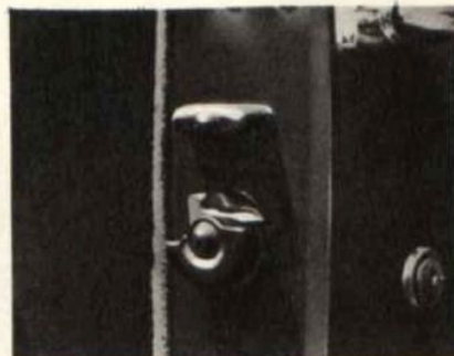
Nash doors shut with one finger. This rotary door latch catches and holds securely. New door stay check holds the door wide open, when desired.
