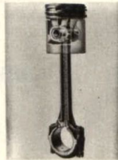
Every cylinder and piston pin is continuously lubricated under full pressure.
