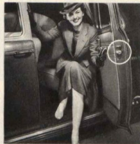
Two new safety features. She steps on a skidproof concealed running board and opens a door with a new rotary latch.
