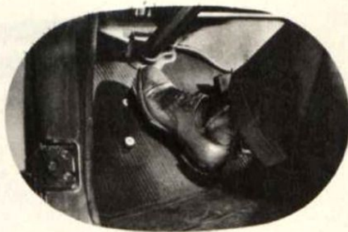
Step on the clutch and the engine starts. This clutch pedal starter disengages the transmission and prevents false starts. The battery never turns the gears over in cold, stiff grease.
