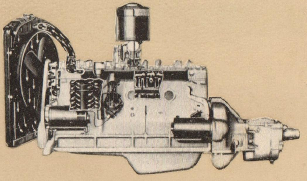
ALL-WEATHER TEMPERATURE CONTROL Assures efficient operation by means of pressure cooling, full-length water jackets, gusher valve cooling, water recirculation and automatic thermostatic temperature control.
