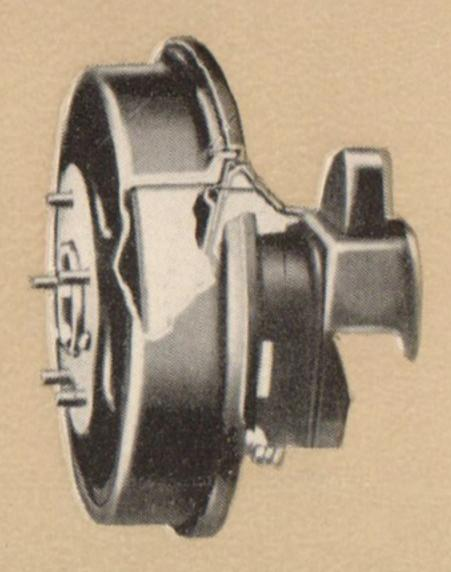
THE CONTROLLING "Self-energizing" principle used in Pontiac's Hydraulic Brakes transforms a light pressure on the brake pedals into a smooth, powerful stopping force. The emergency brake is mechanical and separate from the service brakes.
