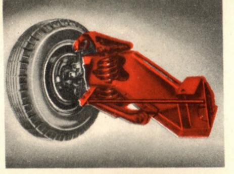
springing, hydraulic telescopic-mounted shock absorbers, stabilizer bar minimizes roll on curves.
