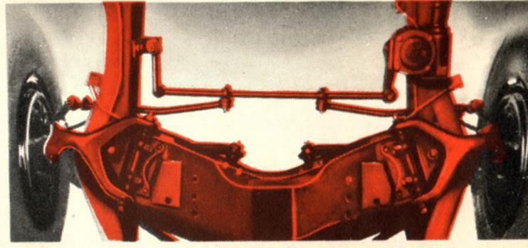
symmetrical balanced steering linkage has expertly engineered leverage for easier, safer, more efficient steering. True finger-tip ease in parking.
