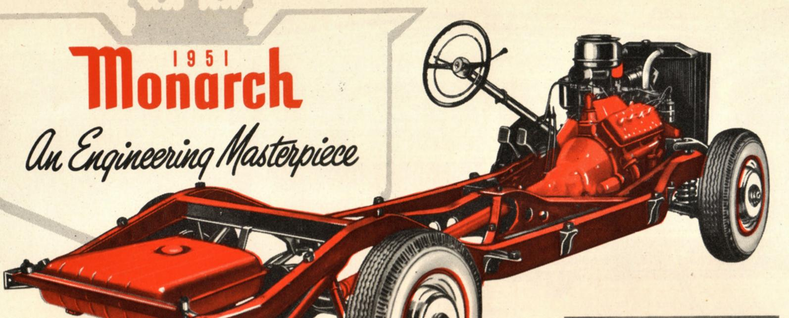
THE MONARCH 1951 CHASSIS is solid, sturdy—engineered for extra rigidity and strength, achieved by X-type frame design with K-type reinforcements. Frame joints are welded and cold-riveted for greater strength. Side rails are specially constructed to withstand strain, tension; they are wide, deep, strong. Your Monarch is built to stand the "gaff" in hardest service—with a chassis that brings you famous Hotchkiss Drive and many other proved advancements for riding comfort and ease of control.
