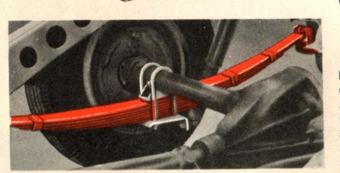
REAR SUSPENSION on two extra-long, semi-elliptic springs with "Sea-Leg" mounted shock absorbers means a superior ride on all roads. Full-length wax impregnated liners provide a permanent lubrication.
