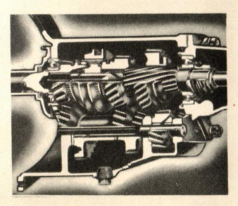
type synchronizers, provides smooth, quiet shifting. Silent-type helical gears are extratough, with wide teeth for strength and longer life.
