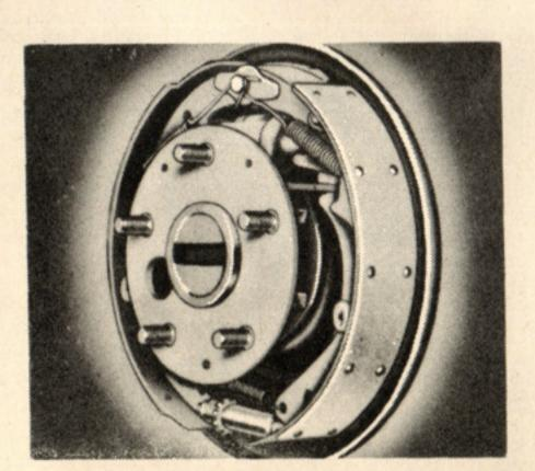
SELF ENERGIZING BRAKES, Duo-Servo type—hydraulic operation—less pedal pressure.
