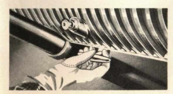
ently located near steering column—permits Overdrive to be locked-out when not desired.
