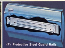
(F) Protective Steel Guard Rails
