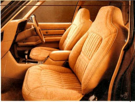
Statesman SL/E seats are trimmed with rich velour facings over full foam construction for driver and passenger comfort.
