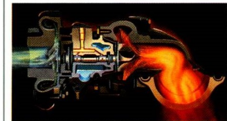
▲ Daytona Turbo Z gets its urge from one of the industry's most advanced turbo-charged engines. Chrysler/Bosch electronic fuel injection and a micro-processor-managed boost control allow transient over-boost for those critical initial seconds of acceleration. Water-cooled turbine bearings ensure reliability—so much so that Chrysler can confidently back the turbocharger and the turbo-charged engine with its full 5 year/80,000 kilometre powertrain warranty. (See back page for details.)
