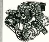
1.6-liter (97.1 CID) four-cylinder engine: 64 hp @ 4,800 rpm; 87 lb-ft torque @ 2,800 rpm.*
