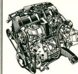
2.2-liter (135 CID) Trans-4 engine: 96 hp @ 5,200 rpm; 119 lb-ft torque @ 3,200 rpm.
