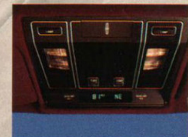
Overhead console (above) features map lights, warning lamps, an electronic compass and an outside tempera- ture display.
