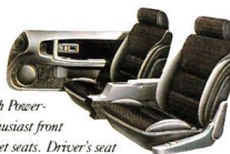
Cloth Enthusiast front bucket seats. Both seats feature adjustable head restraints and seatback recliners. Driver's seat includes power adjustments for lumbar and seatback wings. Standard Shelby, ES Turbo, optional Daytona ES (requires V6 Performance Package).
