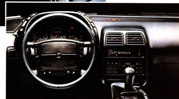
Complete electromechanical analogue instrumentation keeps you informed of all vital functions including voltage, oil pressure, water temperature and vacuum/turbo-boost.
