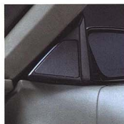
▲ Two high-frequency speakers, mounted on the side mirror interior panels, "lift" the sound image for realistic, orchestrated sound.
