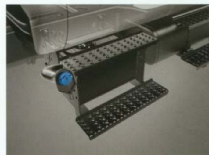
Crew Cab Diesels can get a 38-litre DEF tank option mounted under the cab on the passenger side.
