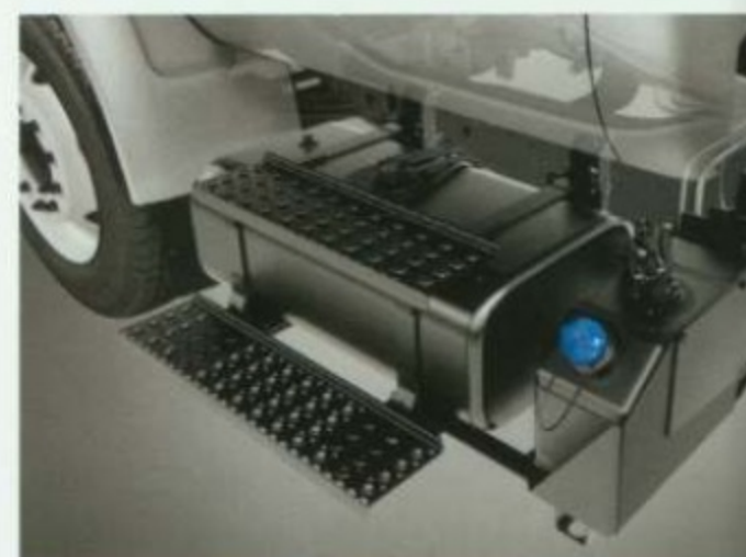
Regular Cab Diesels can get a 132-litre fuel tank and 19-litre DEF tank option mounted under the cab on the driver's side for a clean CA.
