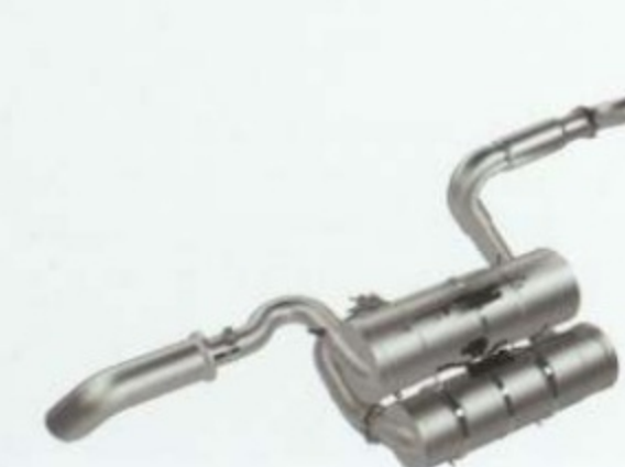
Under-cab horizontal switchback exhaust system 1 is another option we offer to help make your upfits easy and cost-effective.
