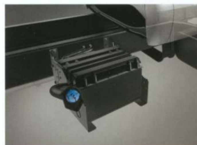
Regular Cab/SuperCab Diesels can get a 38-litre DEF tank option mounted outside the frame rails, behind the cab on the passenger side.
