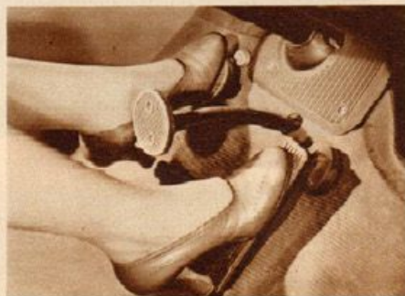
You start this Champion with ease and certainty! The starter button is located beneath the clutch pedal and goes into action when the pedal is all the way down. This ease of starting is just one of many of this new Studebaker's conveniences for simplifying your driving.
