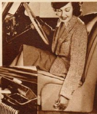
You can adjust the front seat 3½ inches simply by lifting a lever conveniently located at the lower left of the driving seat. Whether you're short, medium or tall, driving comfort in this Champion is extraordinary.
