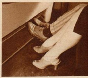
This Champion's hypoid axle assures a flat floor. And, of course, the hypoid gearing means rear axle action that's as silent as a watch. Hypoid gear furthermore excels the conventional gear set-up in its space-saving possibilities. It permits the use of an underslung axle and a low floor level, so that the rear seat passengers get the benefits of a flat floor and increased leg room. Space under the front seat provides extra toe room.
