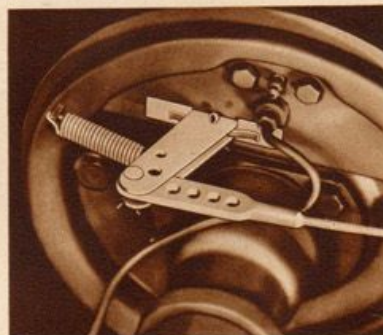
A separate parking brake system that operates by a pull on a lever under the instrument panel gives you an extra factor of safety. It operates by mechanical action on the rear wheels independent of the Champion's efficient hydraulic system.
