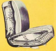
"Cushioned Comfort" for the driver, too. Driver's seat is built for long lasting comfort, with a foam rubber cushion over new non-sag springs. Adjustable to individual driver's comfort. Auxiliary seat optional at extra cost.
