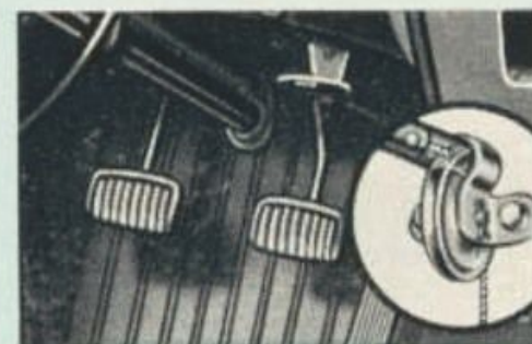
Hand brake cable reverses direction by running back over a free-turning pulley for easier action and longer life.
