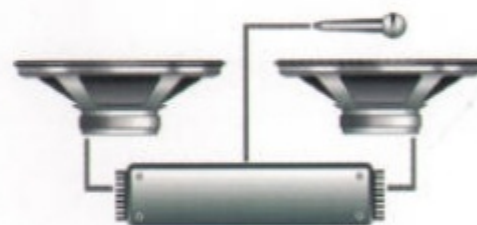
The Acoustic Feedback Sound System uses a microphone within the rear speakers that actually listens to the sound and corrects any distortion it detects.
