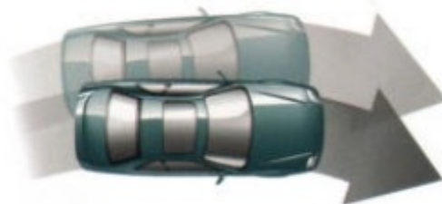
The Active Torque Transfer System minimizes understeer and helps the Prelude Type SH track tight through curves.
