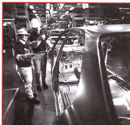
Highly accurate body assembly and laser welding contribute to Avalon's sophisticated appearance
