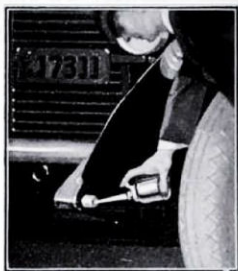
The car is easily and effectively lubricated by means of patented oil cups
