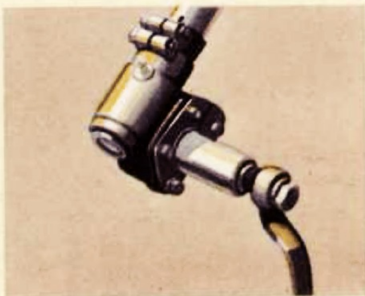
New Easier Steering —A new worm-and-sector steering gear, with 12 to 1 gear ratio and tapered roller bearings, permits easy turning, parking and steering.
