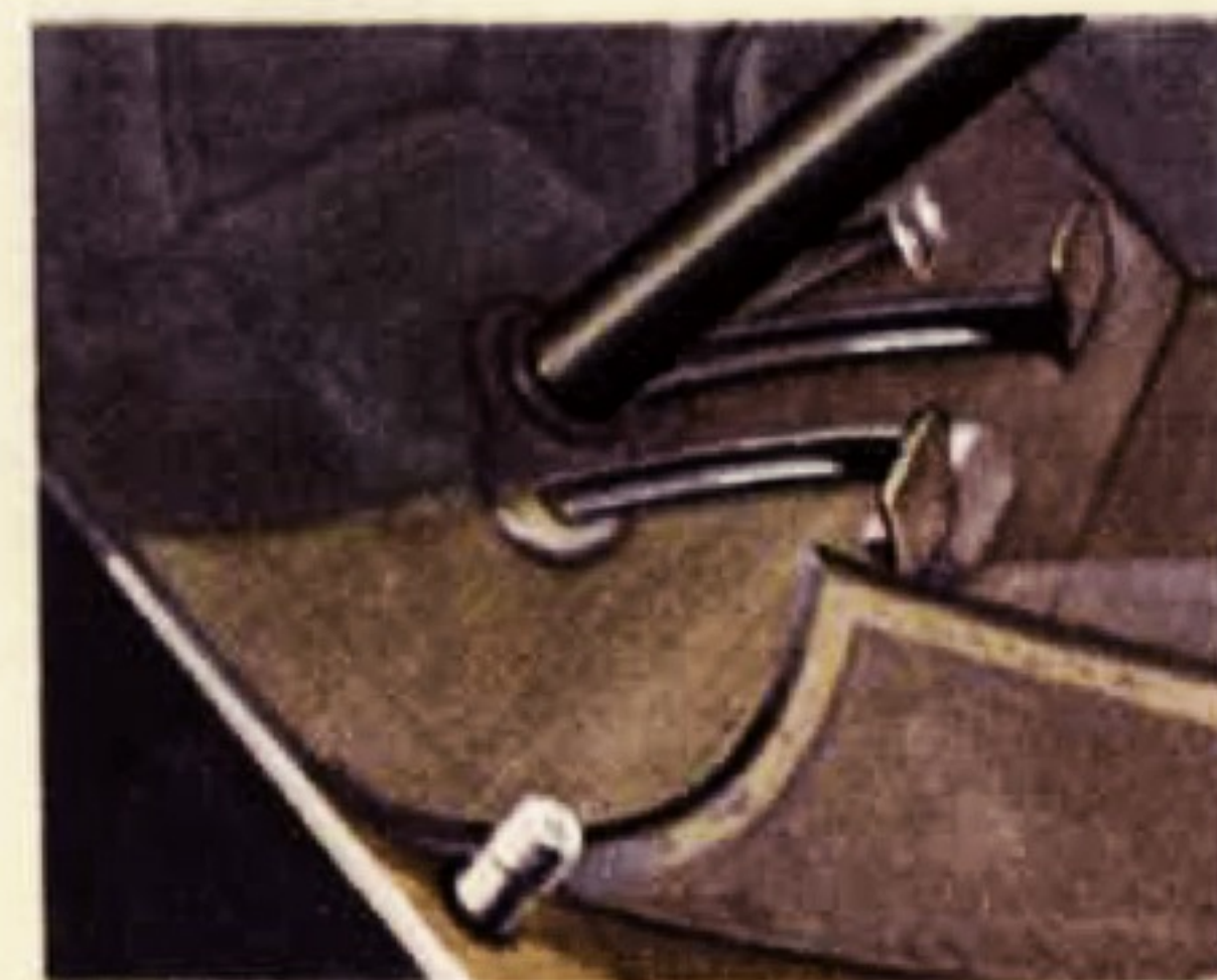
New Dash Insulation —Special insulation material has been installed on the dash and beneath the front floor mat to assure greater comfort for driver and passengers, both winter and summer.
