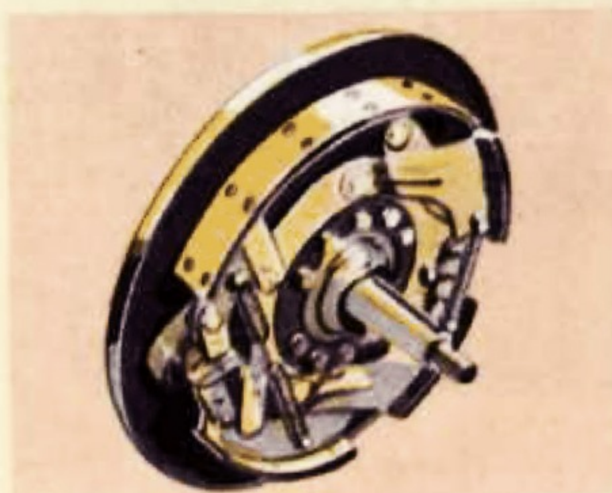
Fully Enclosed 4-Wheel Brakes —The big, powerful 4-wheel brakes of the Chevrolet Six are fully enclosed, positive in action—and equipped with an especially durable moulded brake lining.
