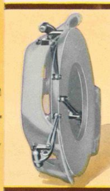
The synchronized all-quiet transmission provides a more convenient change of gears by a shorter movement of the shifter lever. Improvements in the semi-centrifugal clutch make its engagement even softer and smoother
