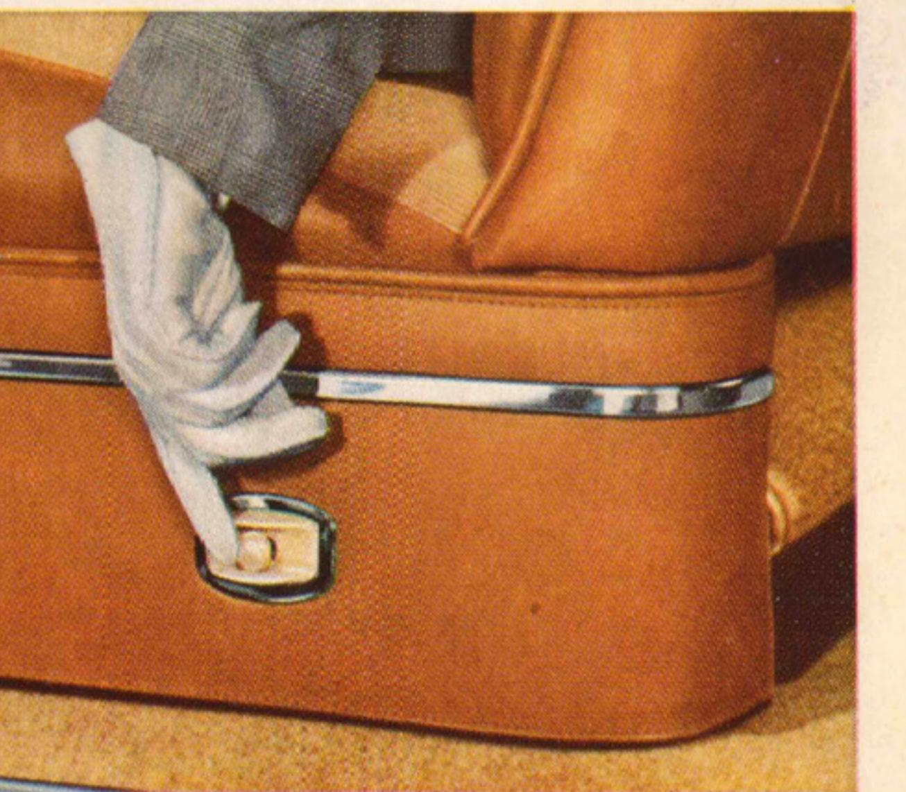
**Prest-O-justment!** That's how easy it is to adjust the power-operated front seat. As the seat moves to the front, it rises and tilts slightly forward, to maintain restful back support and perfect vision. Seat cushions are padded with foam rubber. The swing-aside seat-backs make it an easy step to the roomy rear compartment.
