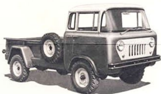
'JEEP' FC-170 TRUCK carries 3,510 pounds of cargo in the pick-up model, and 3,277 pounds in the platform-stake model, thanks to Forward Control design. Single control transfer case lever shifts quickly between 2- and 4-wheel drive. Six-cylinder, L-Head engine. Dual wheel, 8,000lb. G.V.W. option. (Lighter Forward Control Model FC-150 also available.)
