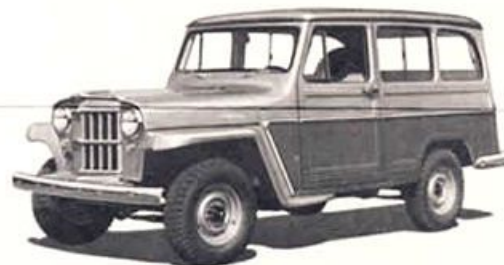
'JEEP' 4WD UTILITY WAGON carries six passengers or a half-ton of cargo. All-purpose, business-pleasure vehicle. Low initial cost, inexpensive operation and upkeep. Piano-hinged tailgate opens to 39½ in. by 58½ in. Choice of engines.
