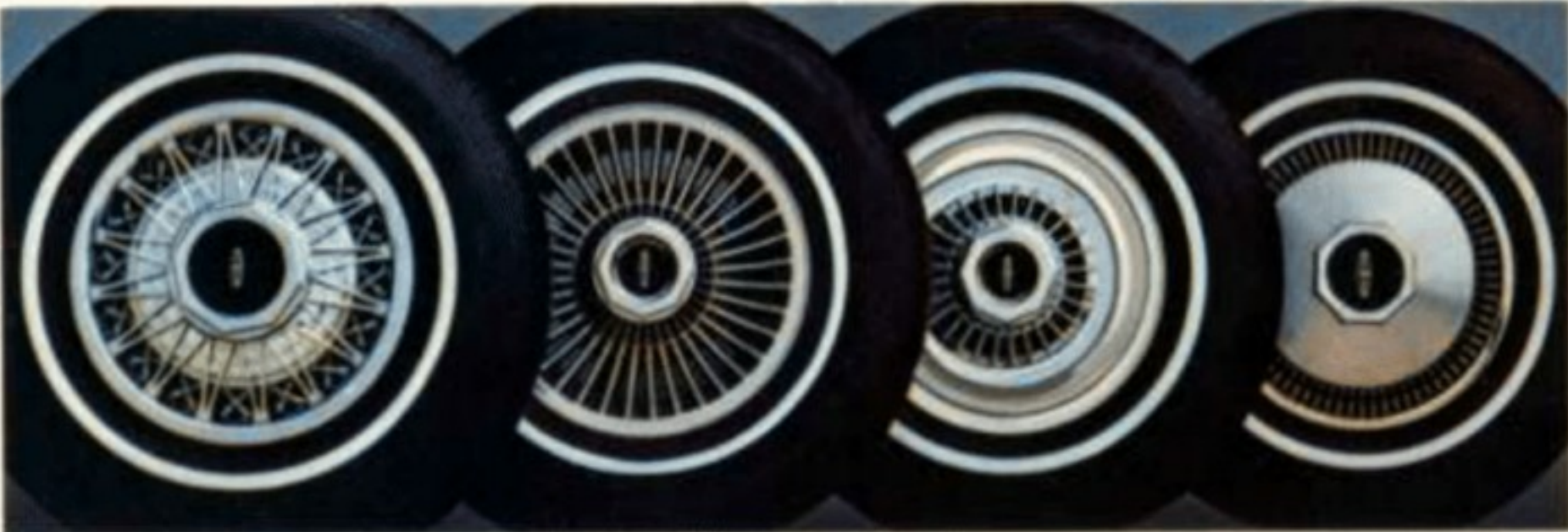
Illustrated left to right optional wire wheel cover, turbine-style cast aluminum wheel, forged aluminum wheel and standard wheel cover.
