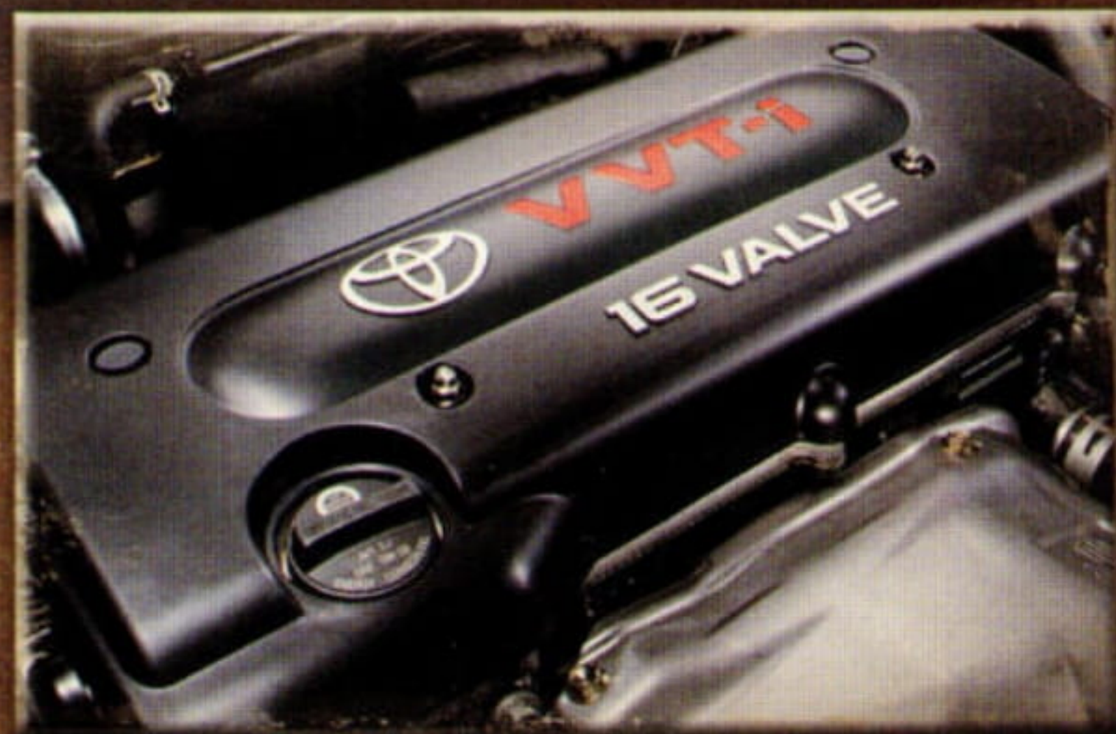
2.4-liter DOHC 16-valve VVT-i 4-cylinder.
