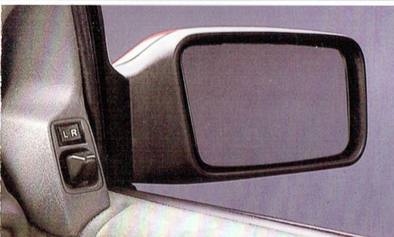
*Exterior rear view mirrors are electrically adjusted.*
