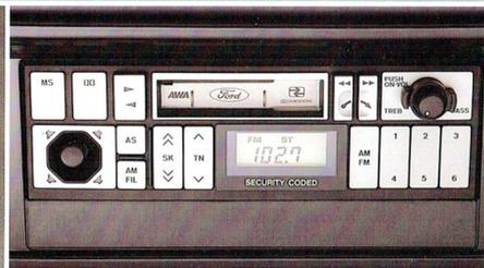
*AM/FM stereo radio-cassette with Dolby sound, auto scan memory and new security-coded theft deterrent system.*
