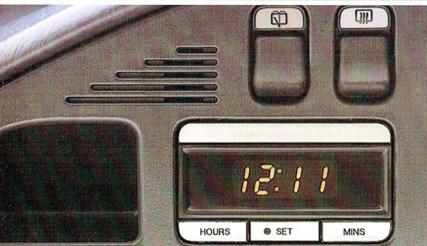
*Rear window washer/wiper, and demister switches plus a clear digital clock are conveniently located.*
