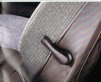
*Driver's seat has fore/aft, cushion height and backrest rake adjustments, plus 4-position lumbar support and adjustable headrests.*
