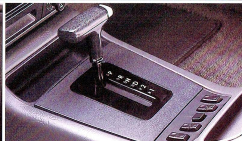
*Centre console includes power window controls. A lockout switch deactivates the rear door windows and cigar lighters.*
