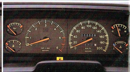
*Comprehensive instrumentation includes speedometer, tachometer, oil pressure, fuel, temperature, battery gauges.*
