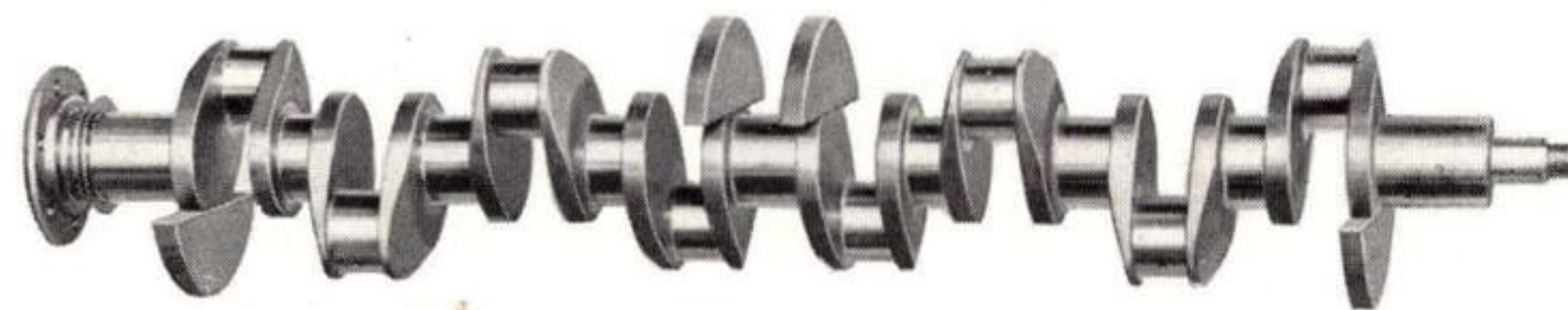
THE NEW COUNTERBALANCED CRANKSHAFT FOR THE PACKARD EIGHT
