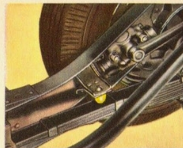
Auxiliary rear spring bumpers prevent possible shock caused by springs striking through.
