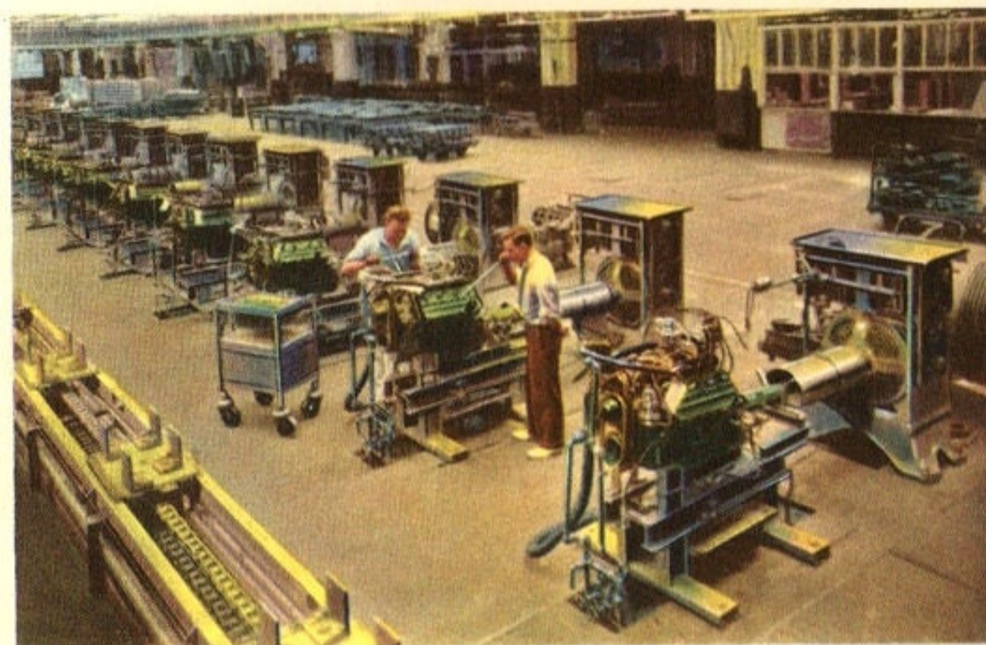
Engines are run continuously for many hours. Smoothness, quietness, and compression are checked and rechecked by accurate machines.
