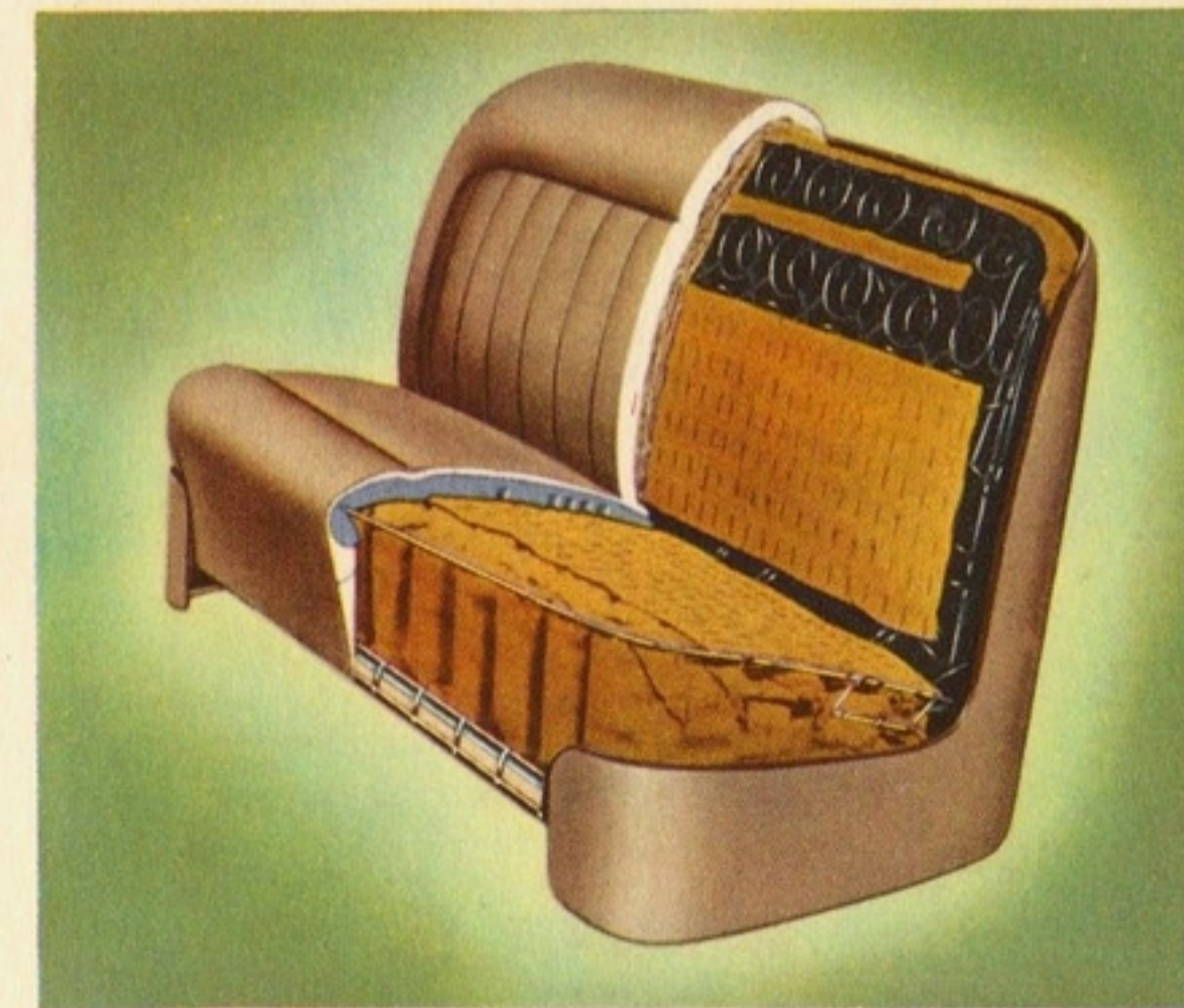
Cadillac's combination rubber and cloth padding seat construction makes for exceptional softness and coolness.
