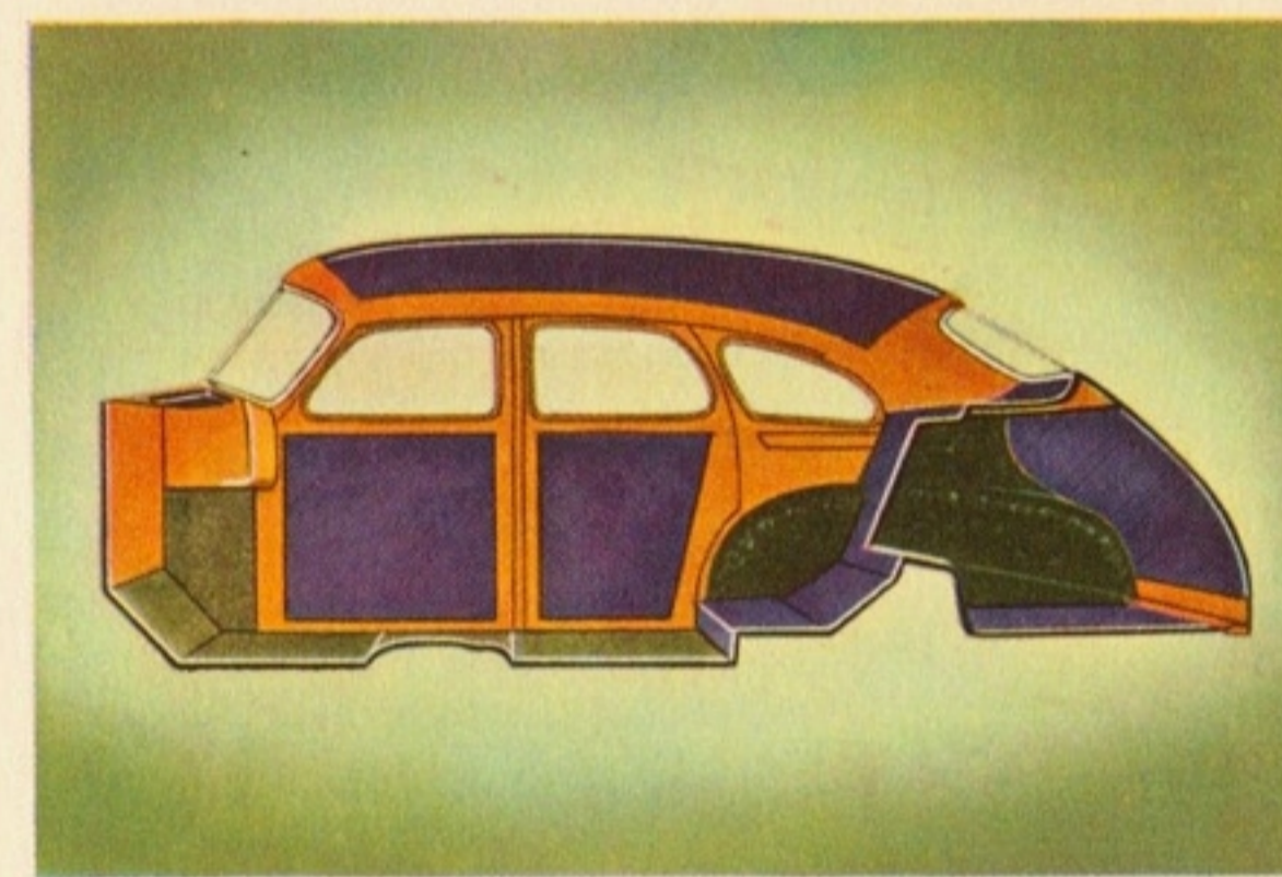
Body insulation, further improved this year, results in a noticeably quieter body. Six insulating materials are used.
