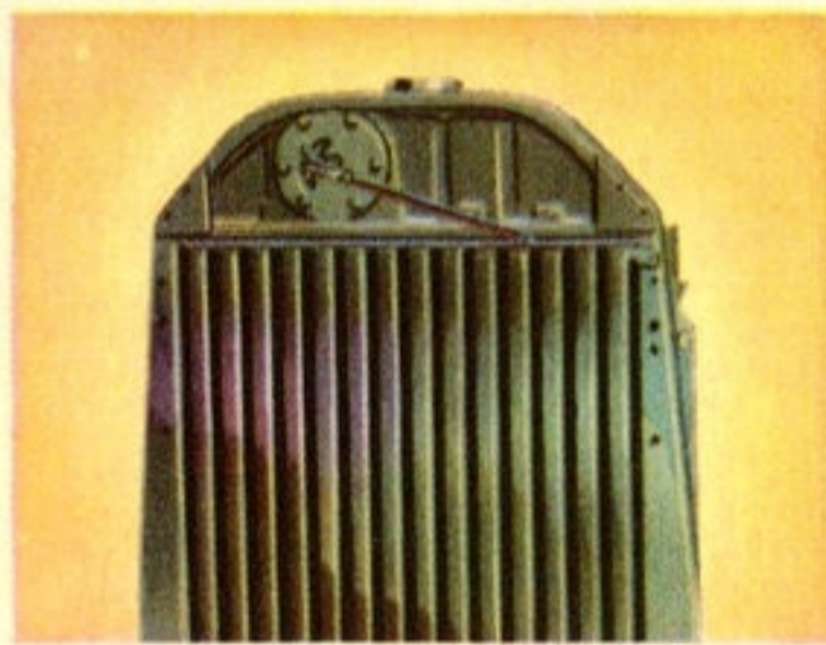
Automatic radiator shutters maintain higher underhood temperatures. Gasoline vaporizes more completely.
