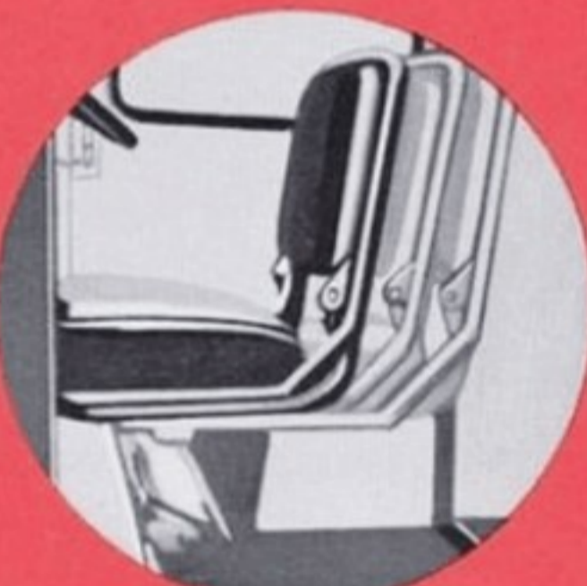
ADJUSTABLE SEAT moves forward or back, up or down. Folds under the steering wheel for easy access to the cargo area.
