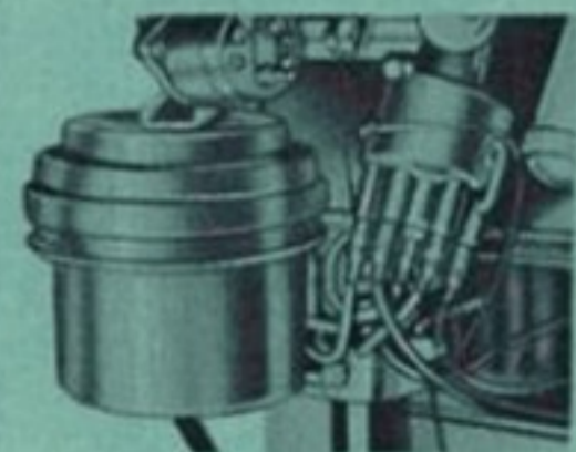
OIL-BATH AIR CLEANER assures that only clean air enters the engine. It efficiently removes abrasive dust that causes engine wear. Here is a valuable feature that other truckers pay extra for . . . yet it's standard in Chevy!
