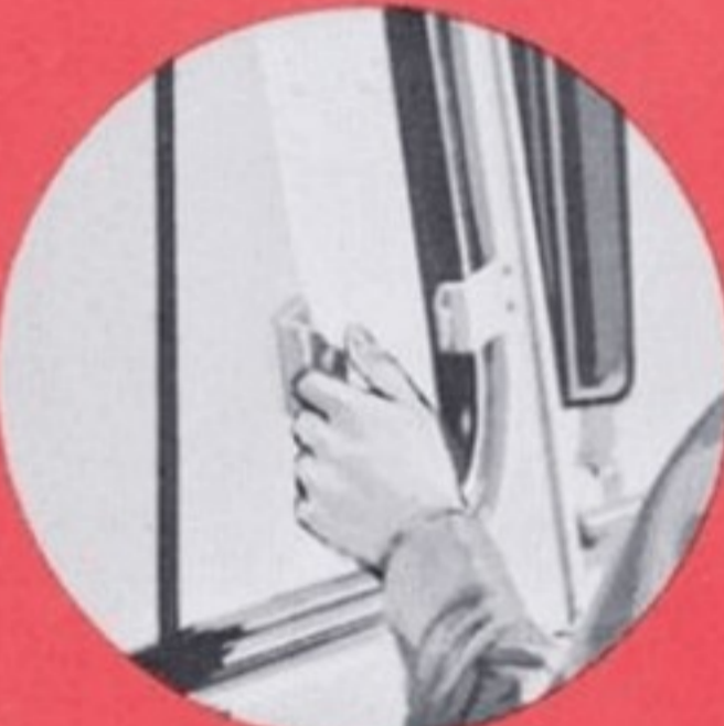
SLIDING WINDOW , located on driver's side, opens easily for ventilating or signalling. When shut, it is leakproof.
