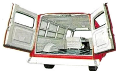
EXTRA LOADING EASE —Big wide rear doors open from floor to roof for easy access to the load compartment. Telescoping door checks stop doors automatically at 90 or 180 degrees. And Chevy's lower to the ground chassis design makes it easier than ever to pack in the payload.
