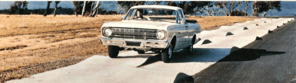
Above: The "Body-Twist Road" — a brutal test of body tightness and structural strength. Durability of body structure and chassis components never got a more rugged test. Tests were run for mile after
