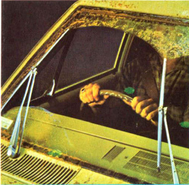
Holden Articulated Windscreen Wipers eliminate driver's "blind spot".
