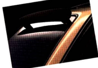
Rear window air deflector.
