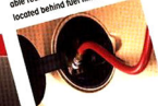
Control valve for available inflatable rear shocks is conveniently located behind fuel filler door.
