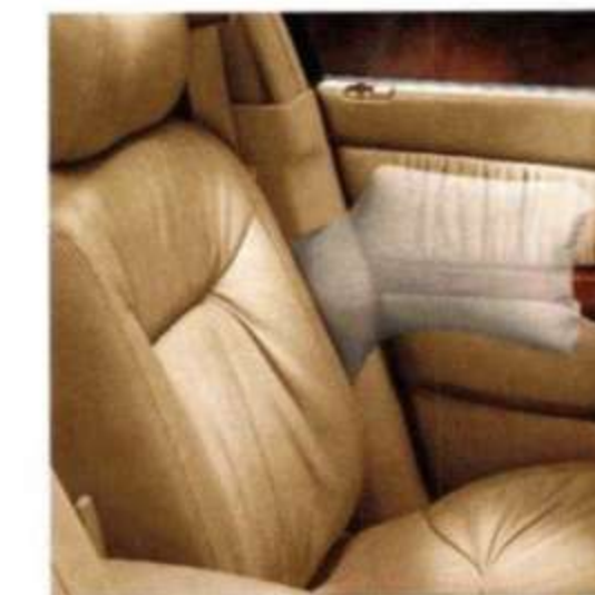
Front Side Air Bags are featured in each front seat for enhanced protection from side impacts. Sensors in the front passenger's seat prevent the air bag from deploying if a child or small adult is out of position.
