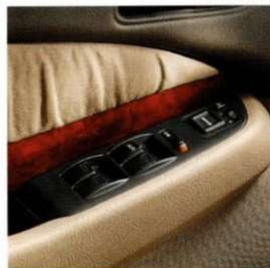
An Ergonomically-Designed Control Panel, located in the driver's side front-door handle, keeps power window and mirror controls comfortably within reach.
