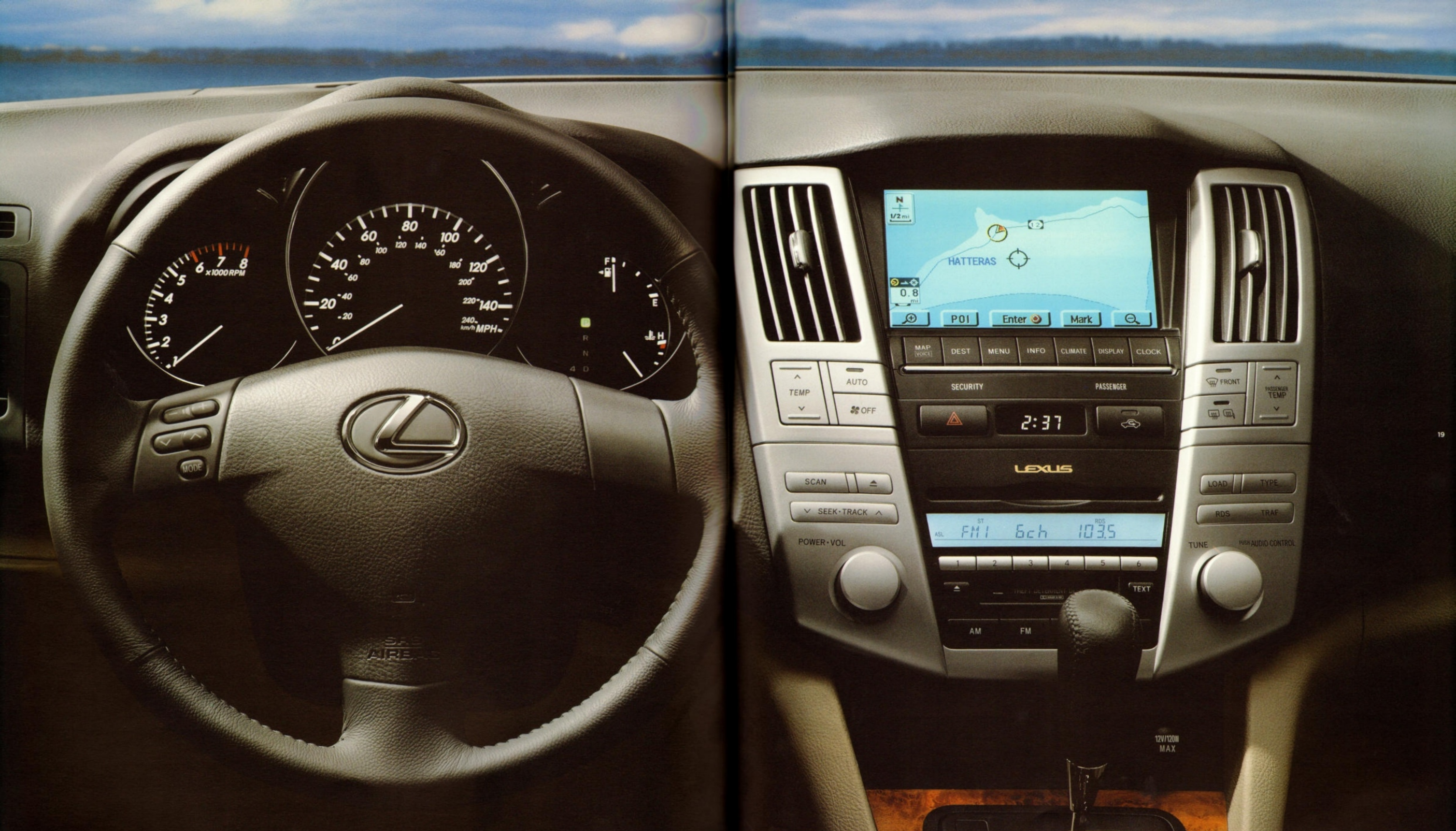
The redesigned interior includes electroluminescent meter instrumentation in a three-pod layout, a seven-inch-wide, liquid-crystal information screen and handy steering-wheel audio controls.
