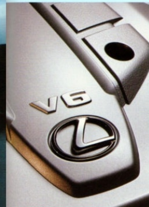
GS 300— 245-hp V6 with dual Variable Valve Timing with intelligence (VVT-i) and direct injection.
