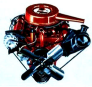
Super Rocket V8. New 2-barrel carb. 310 hp, 450 lb.-ft. torque, 425-cu-in. 10.25-to-1. Premium fuel. Standard on Delta and Dynamic 88. 300 hp regular fuel available, no extra cost, on Dynamic 88 only.
