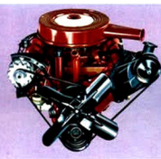
Starfire V8. Quadrajet Carburetor. High-lift camshaft. 425-cu-in. 375 hp, 470 lb.-ft. torque, 10.5-to-1 compression ratio. Premium fuel. Available on all Ninety-Eight and Delta 88 models at extra cost.
