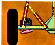
Twin-Triangle Rear Suspension incorporates four control arms, using triangular geometry, to help reduce rear-end squat. Wide pivot points and a lightweight axle also help to keep every Olds on the level.
