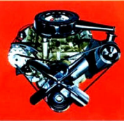
Jetfire Rocket V8. Biggest V8 in its class. 330-cu-in. displacement. 290 hp, 335 lb.-ft. torque, 9.6-to-1 compression. Regular fuel. Available on F-85 Deluxe. Standard on Vista-Cruiser.
