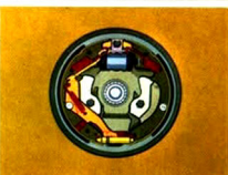
Air-Scoop Brakes have wide flange that sweeps up air to dissipate heat. Thick linings reduce wear. Large lining areas, plus organic compounds, aid stopping power. All brakes are self-adjusting, self-energizing.
