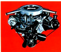
Toronado Rocket V8. Oldsmobile's top-performing Rocket. Twin-snorkel air cleaner. Quadrajet Carb. 425-cu-in. 385 hp, 475 lb.-ft. torque, 10.5-to-1 compression. Standard on both Toronado models.
