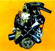
Action-Line 6. New in-line design delivers power efficiently, improves fuel economy, durability. 250-cu-in. displacement. 155 hp, 240 lb.-ft. torque, 8.5-to-1 compression. Regular fuel. F-85 Deluxe only.
