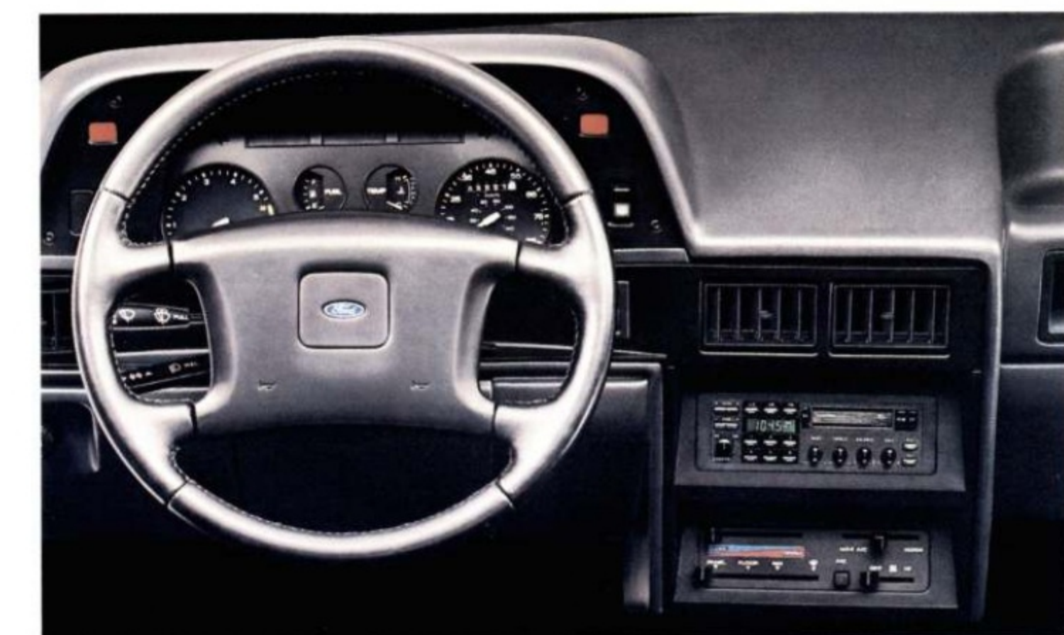
Right: The Escort GT instrument cluster includes a tachometer, engine temperature gauge, and trip odometer.
