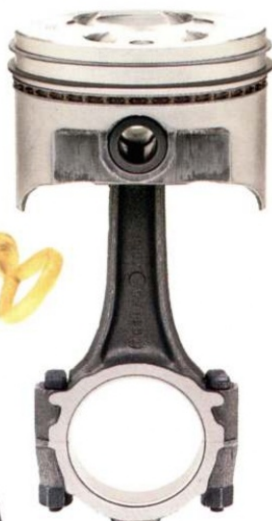
The 5.0L uses forged aluminum alloy pistons for light weight and good heat dissipation. The connecting rods are forged steel for strength.
